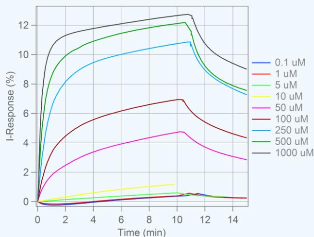
Agile Plus software-generated overlay plot displays a full kinetic characterization using COOH Agile biosensors. A concentration series of small molecule SPD304 is measured against immobilized TNF $\alpha$ , a cell signaling protein used as a therapeutic target. These curves show the concentration dependence of the biomolecular interaction, and the evaluation software provides  $k_{on}$ ,  $k_{off}$ , and  $K_D$ .
